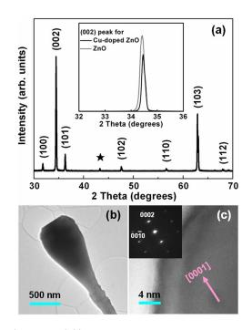
FIG. 1. (Color online) (a) XRD pattern of the Cu-doped ZnO sample. The star indicates a peak from the Au catalyst. The inset is the (002) peaks of the undoped and the Cu-doped samples. (b) Low-resolution and (c) high-resolution TEM images of a nanonail. The inset of (c) shows a SAED pattern.
