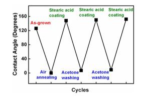
FIG. 4. (Color online) Reversible transitions between superhydrophilicity induced by air annealing and superhydrophobicity induced by stearic acid coating.
