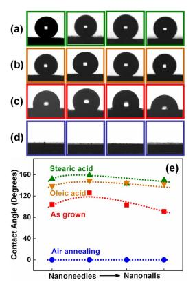
FIG. 3. (Color online) Shapes of water droplets photographed on four equally spaced positions as depicted in Fig. 2 for (a) stearic acid treated, (b) oleic acid treated, (c) as-grown, and (d) air-annealed samples. The corresponding CA were plotted in (e).
