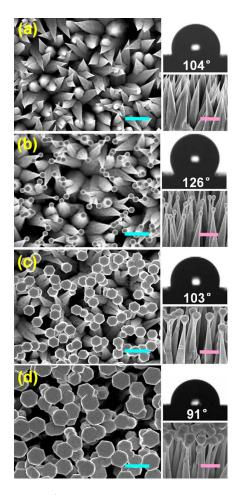
FIG. 2. (Color online) FESEM top and cross-section views of (a) nanoneedles and [(b-d)] nanonails of Cu-doped ZnO grown on silicon substrates. Photographs of water droplets and CA measured on each position are shown at the top right corners. The scale bars represent 5  $\mu$ m in length.
